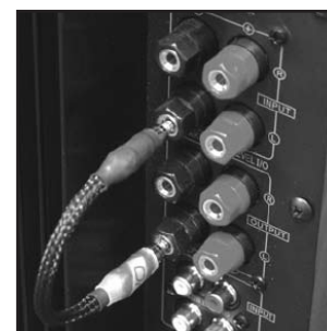
Looping the left negative input to the left negative output will help in any situation where a powerline "hum" is present
