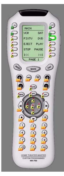
In this example, a system with a VCR, a DVD player, a Satellite receiver, a TV and a surround sound receiver has all of the basic commands on one page. No button ever changes its function. For some users this is simpler to understand and they do not require the hobbyist functions.
