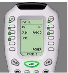
**2** On the new device's first page, create a shortcut to each problem component's power command by pulling down the device list, then the command list.
