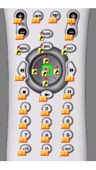
5 Program Power On and Activity Macros as needed. In this example system, there are only two activities (watching VCR or watching SAT), so the only macros are Power On and Off (which actually turn on four components: the TV, the VCR, the Satellite receiver and the surround sound receiver) and the Activity Macros for watching VCR or watching Satellite (which simply switch inputs on the surround sound receiver).
